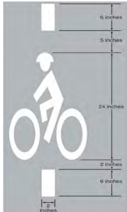
Bicycle detector symbol (CA MUTCD Figure 9C-7)
